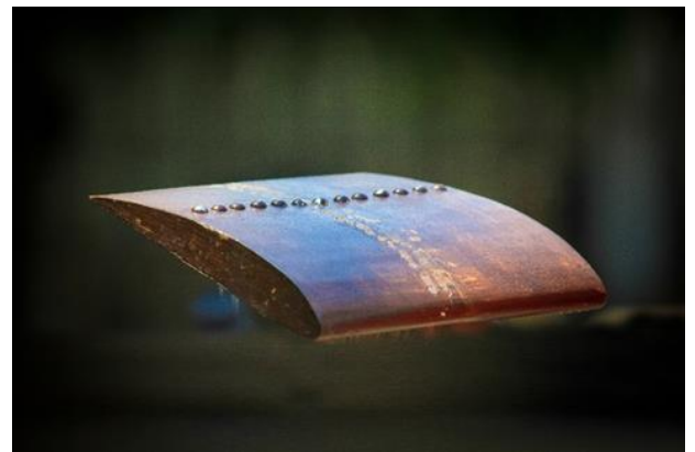
Fig .2(b): Constructed model with outward dimples
