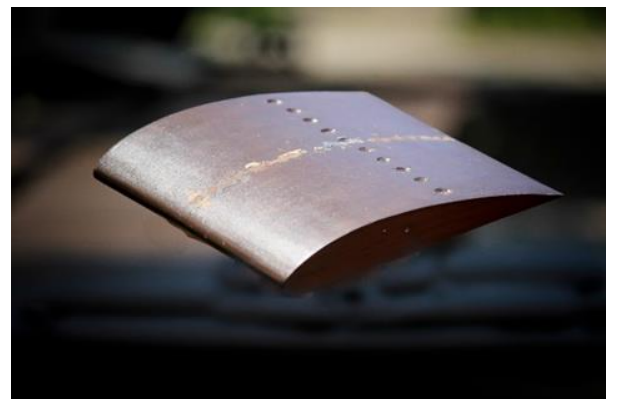
Fig.2(c): Constructed model with inward dimples
